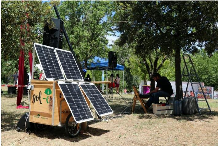
*Sol-ê, EnergÉtica’s device to generate clean electricity in a portable way*
